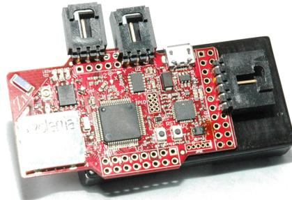
**Figure 2.1:** Zolertia Z1 mote. Picture taken from the Zolertia website.
